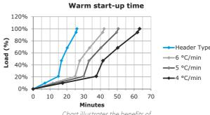
Chart illustrates the benefits of fast (9 °C/min) ramp-up The SGS3 system, which is also securing reliable operation of the Godawari 50MW CSP plant, is developed based on traditional boiler principles (ASME and EN standard header and coil type) not as ordinary heat exchangers (TEMA standard kettle- and shell & tube-type).
